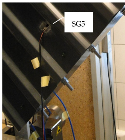
Figure 4. Strain gauge (SG) measurements: (a) scheme of the SG location; (b) SG 5 during the test; (c) SG 1, 2, 3 and 4 during the test.
