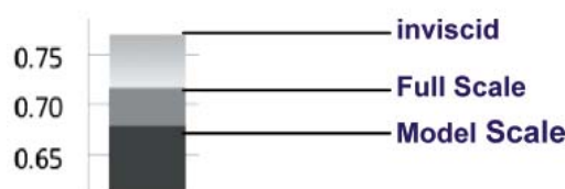
Fig. 4. Illustration of the inviscid propeller concept (left). The model scale efficiency is measured, the estimation and subtraction of model scale surface friction forces gives the in-viscid performance and a guess for full scale friction effects reduces the inviscid efficiency to the full scale efficiency. The diagram on the right holds for propeller 2004 ( D = 0.382m ), operated at 18 Hz ( Re_{0.7} = 2.3 \cdot 10^6 ) in HSVA's large conventional tunnel. Various methods were used to execute the steps explained on the left. For propeller 2004 the full scale efficiency level in the ITTC column (reflecting the application of the ITTC'78 scaling procedure) is hardly visible as it was predicted slightly below model scale efficiency.
