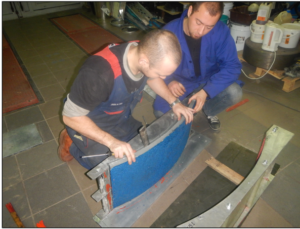
Figure 4: Manufacturing of replica road surfaces
