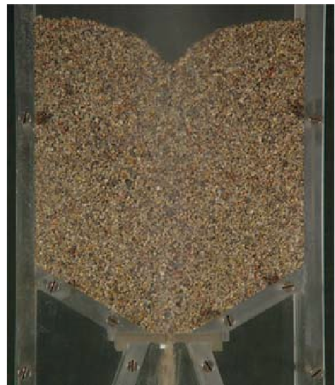
Fig. 8. Model silo with smooth walls: a) mass flow silo, b) funnel flow silo
