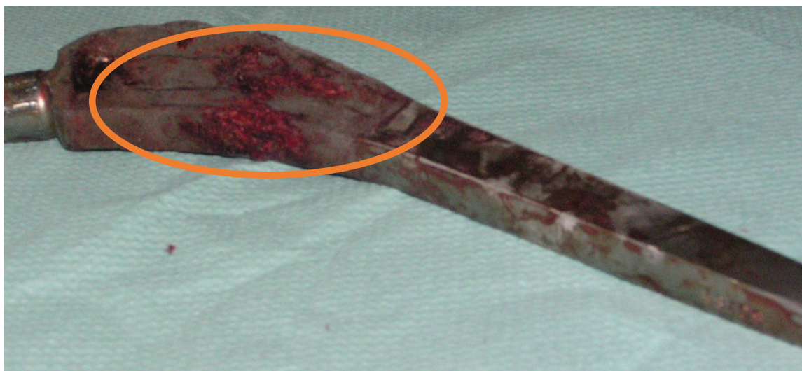
Fig. 3. Endoprosthesis with metallosis
