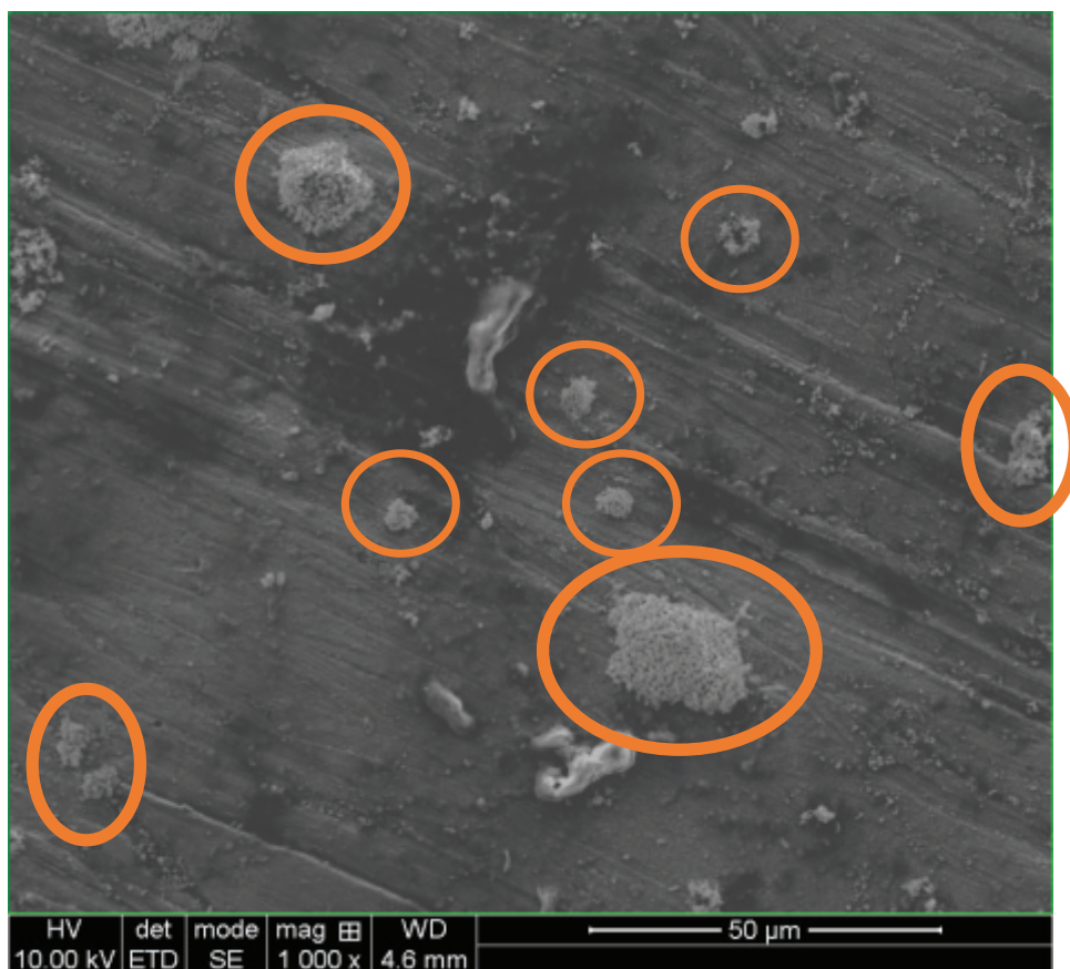
Fig. 6. Biofilm on the surface of the implant
