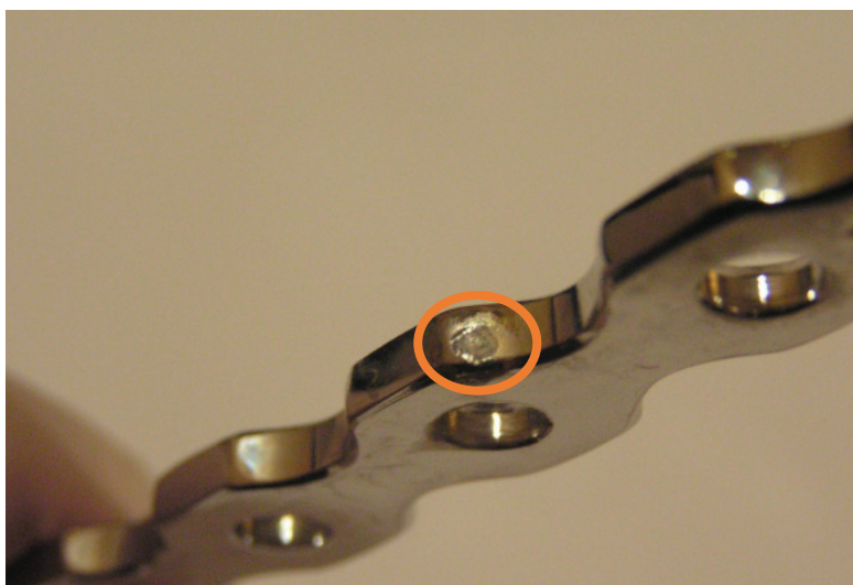
Fig. 4. Plates used for join bones with corrosive focus
