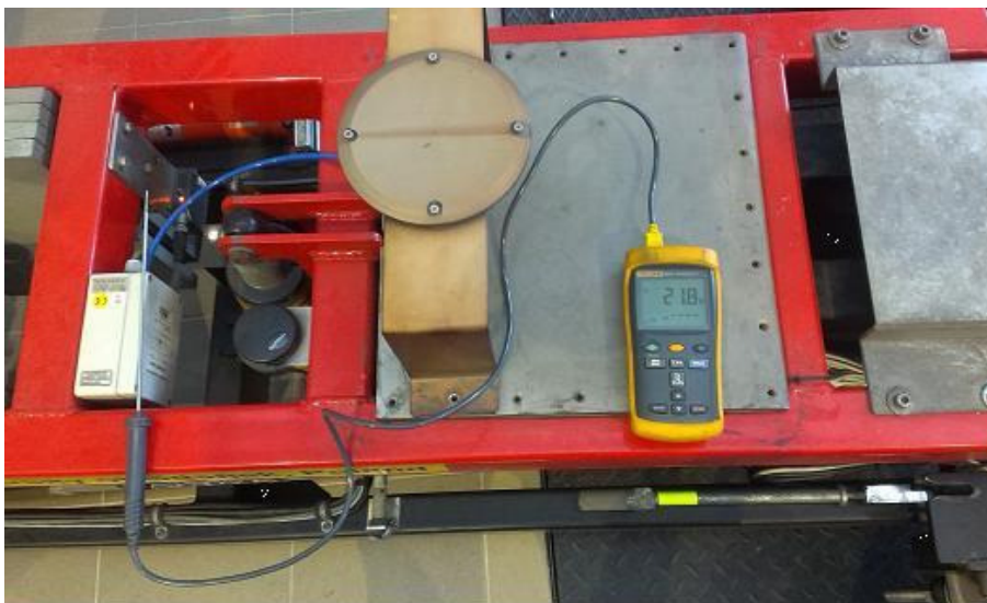
Figure 10. Testing of the temperature sensors (in TUG trailer air temperature sensor is mounted outside the wind protective chamber).
