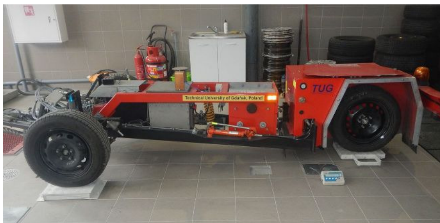
Figure 6. Calibration of R2 Mk.2 trailer - testing tyre load.
