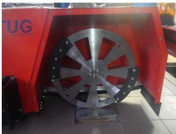
Figure 11. Calibration of R 2 Mk.2 trailer - radius of the test wheel influence.
