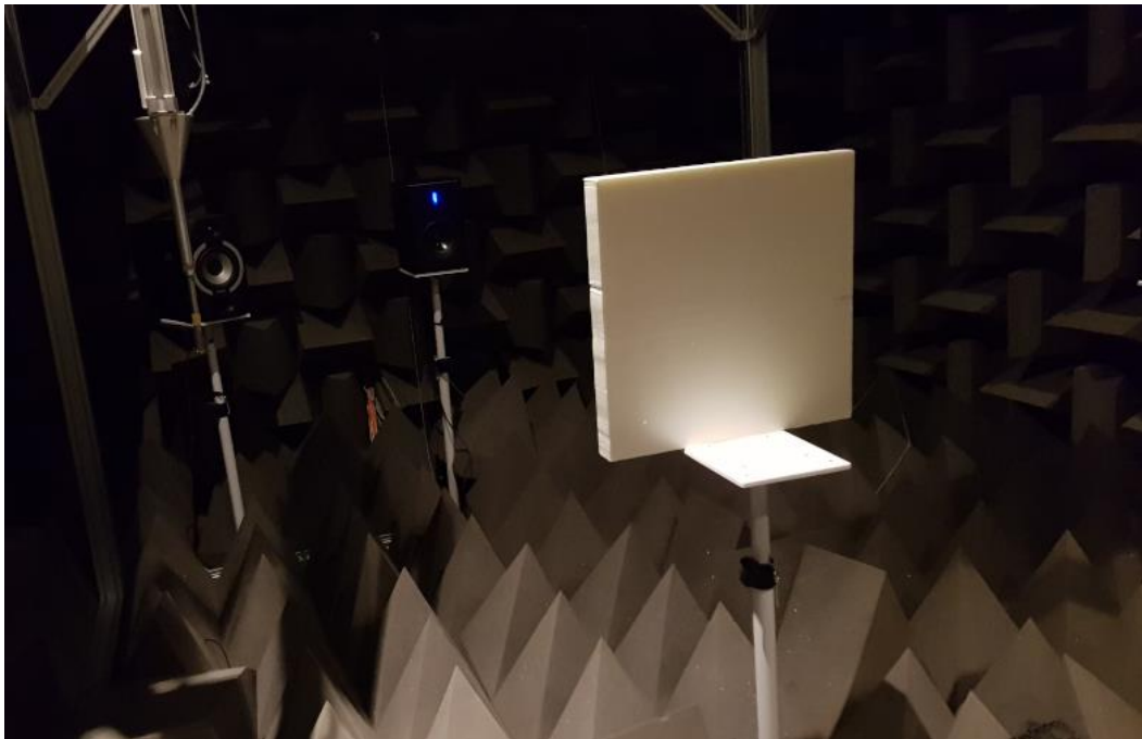
Fig. 6.10 Arrangement of objects in the anechoic chamber to measure the diffusion coefficient of the flat plate. An APS Coax studio monitor used as a sound wave source and Microflow Acoustic Probe used for the measurement are also visible in the picture. Also, parts of the Cartesian robot structure are visible on the sides of the measurement area.
