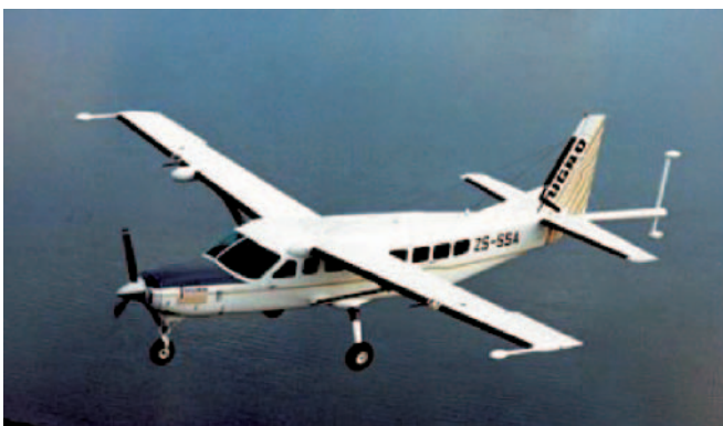
Fig. 12. The magnetic system with a set of magnetometers (the sensors are installed in the tail of the plane and on wings) [14]
