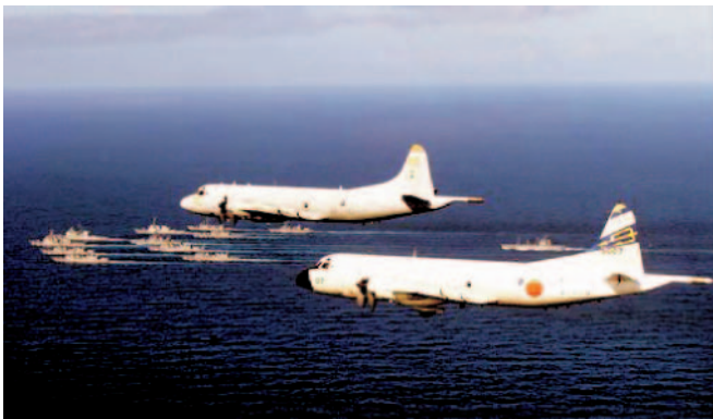
Fig. 11. The military magnetic system with one magnetometer (the sensor is in the tail of the plane)
