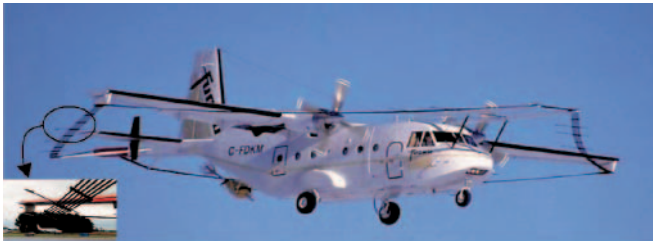
Fig. 3. The GEOTEM electromagnetic system on the plane Casa 212 [4]
