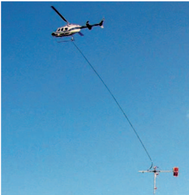
Fig. 16. The magnetic system on a helicopter with the magnetic sensor inside the gondola
