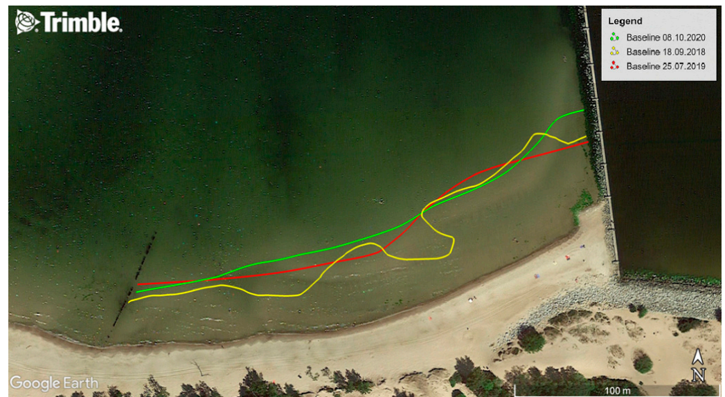
Figure 7. The course of the TSB of the waterbody located at the approach to Górkzi Zachodnie from the Gdańsk Bay measured with the hydrographic method in 2018–2020.
