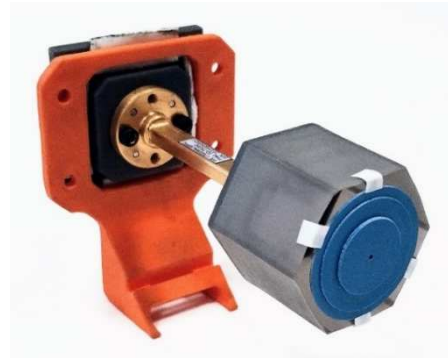
Figure 9. The assembled antenna in a measurement setup, from the left: measurement fixture, WR15 waveguide, 3-D printed spacer and LTCC lens.
