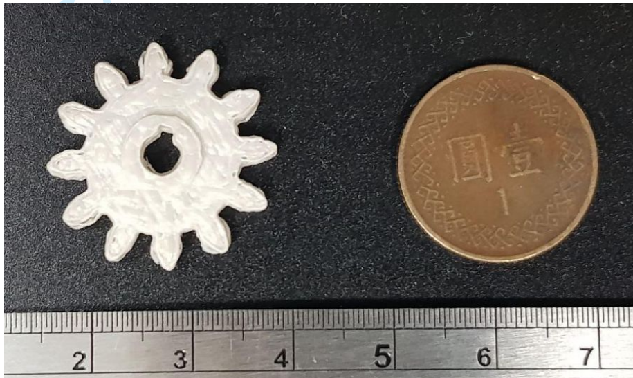
34 35 Figure 15: Demonstration of post-sintered mechanical gear prototype fabricated with zirconia 36 slurry. 37
