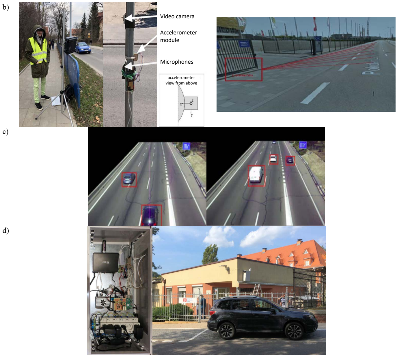
Fig. 3 Block diagram (a), experimental installations for comparative tests of laser, optical and acoustic sensors (b), effects of image processing from a video camera by a deeply trained neural network (c), hardware implementation of an integrated experimental laboratory stand (d)
