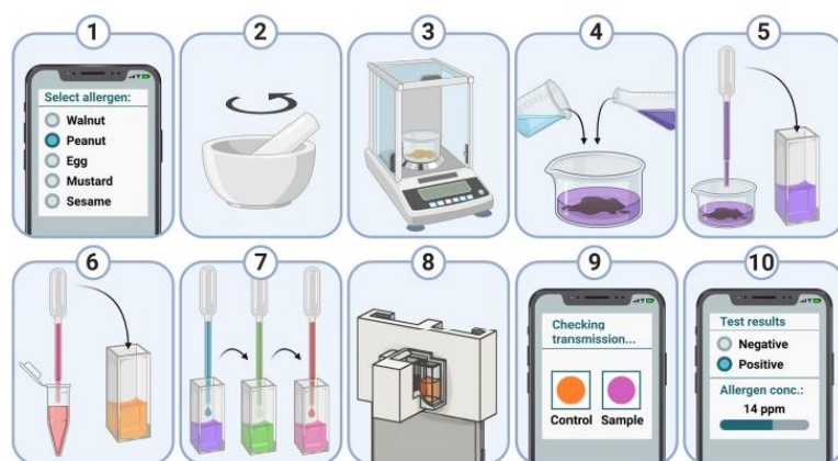
Fig. 4. Procedure for determination of allergens in food samples using a smartphone attachment and colourimetric assays: (1) the allergen of interest is selected in the application; (2) a food sample is finely ground; (3) approx. 5 g of the ground sample is transferred to a vessel; (4) the sample is mixed with water at 60 °C and with extraction solvent; (5) 3 drops of the sample solution is added to the first tube; (6) 3 drops of the control solution are added to the second tube which will act as reference; (7) following a 10 min incubation period, both the test and the control tubes are sequentially rinsed with a conjugate, substrate, and a stop solution, with a wash buffer used in between the rinses; (8, 9) absorbance of both solutions is measured using a dedicated smartphone attachment; (10) the test provides qualitative and quantitative information. Own rendering based on (Coskun et al., 2013).
