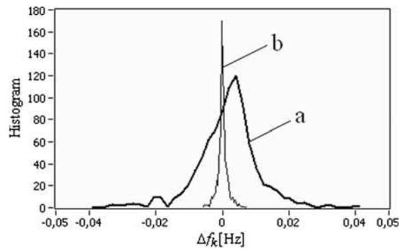
measured frequency, assuming a linear change of frequency  $f = f_0 + a \cdot t + s$  for  $f_0 = 20$  Hz,  $a = 2$  Hz/s,  $s_{\max} = 0.001$  Hz and the even sampling period  $T_S = 100$  ms, where  $s$  is the noise ( $s$  simulates the noise of the measured signal, but also processing errors). Error values were calculated as the difference between the frequency  $f'_k$  obtained from the measurement and value  $f_k$  accepted as true at the time  $t_k$ :  $\Delta f_k = f'_k - f_k$ .
