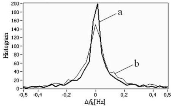
**Fig. 9** Histograms of errors  $\Delta f_k$  distribution for  $f_0 = 20$  Hz,  $f_m = 2$  Hz,  $f_s = 0.3$  Hz,  $s_{\max} = 0.001$  Hz and  $T_S = 20$  ms; **a** frequency determination from last period, **b** frequency determination from two last periods
