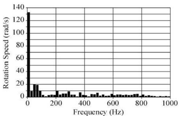
(Fig. 15), and then set a frequency spectrum signal speed of the motor shaft (Fig. 16) with a visible component of a constant value of 133 rad/s and a 50 Hz component of the value of 20 rad/s.
