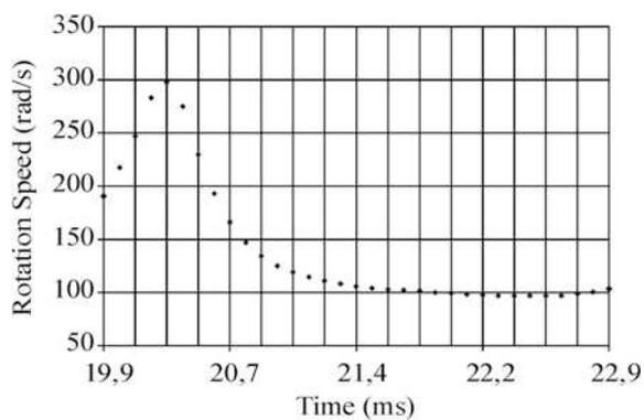
**Fig. 15** Rotation speed evenly sampled converted from Fig. 14 using offline mode method (12)
