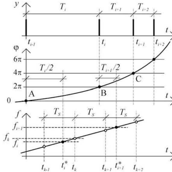
interval  $T_i$ . Therefore, it is reasonable to interpolate in the time interval from the time  $t_i^* = t_{i-1} + T_i/2$  to time  $t_{i+1}^* = t_i + T_{i+1}/2$ , for which the instantaneous frequency takes appropriate values  $f_i = 1/T_i$  and  $f_{i+1} = 1/T_{i+1}$ . Following points  $t_i^*$ ,  $f_i$ :
