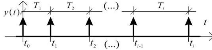
Fig. 2 The idealised frequency-pulse signal
