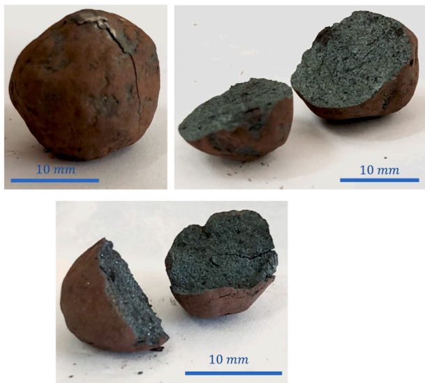
Fig. 11. Pellets aspect after the compression tests.
