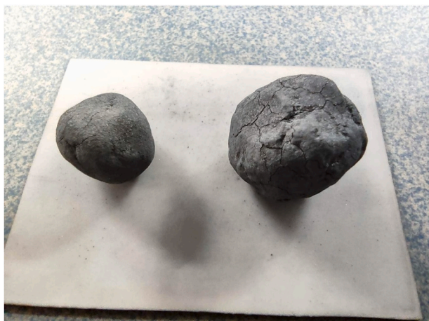
Fig. 13. Pellets reduced in hydrogen at 1000 °C.
