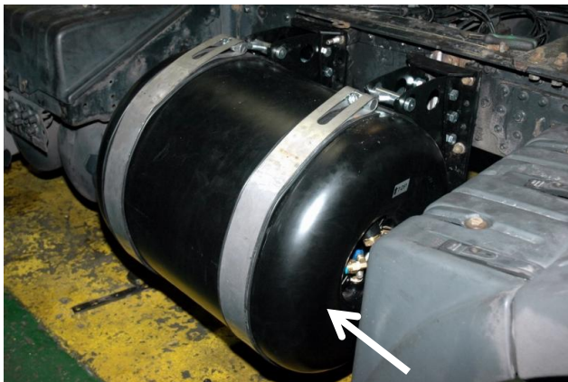
Fig. 3.3. The additional LPG tank in the tractor
