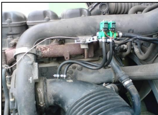
Fig. 3.5. The example of gas valves location and gas inlet in the tractor
