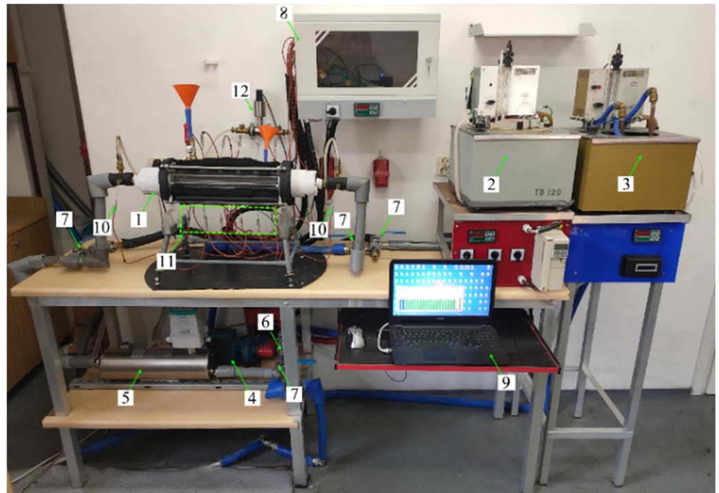
Figure 1. View of the experimental stand: 1—LHSS, 2—hot water thermostat, 3—cold water thermostat, 4—pump, 5—ultrasonic flow meter, 6—needle valve, 7—three-way valve, 8—multiplexer, 9—PC, 10–11—resistance thermometer, 12—pressure difference transducer.
