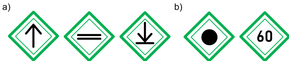
Fig. 7.7. Proposed trackside signs for optimized velocity profile: a) phase change signs for accelerating/cruising, coasting, and decelerating; b) additional signs to be placed with phase change signs: for station and set velocity
