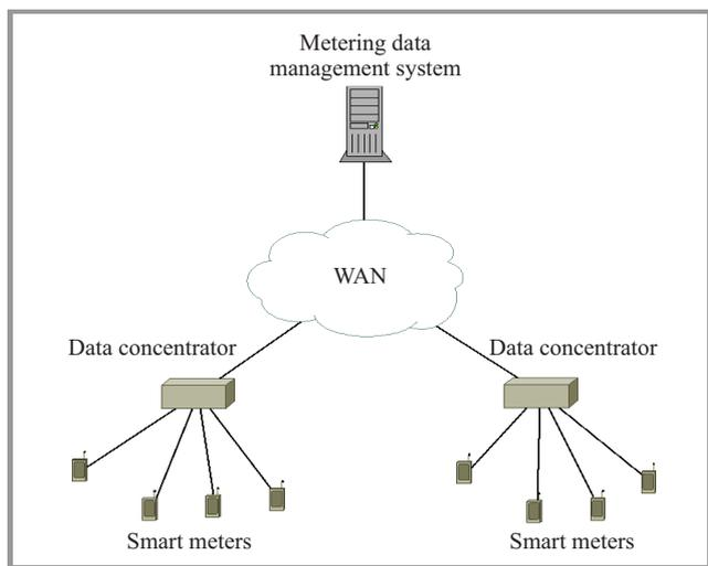
Fig. 2. High-level Advanced Metering Infrastructure diagram.
