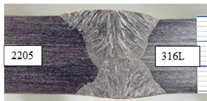
Fig. 2. Macrostructure of dissimilar 2205 – 316L welded joint
