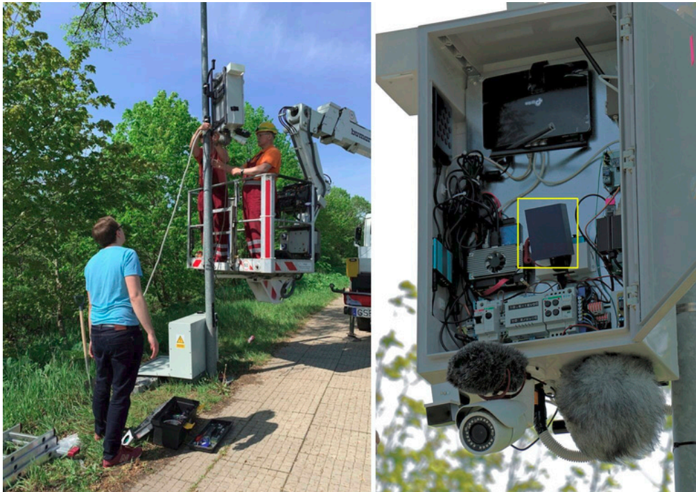
Figure 15. The test system mounted on the site. The Doppler sensor is located inside the box marked with the rectangle, the AVS in a windshield is visible at the bottom right, below the enclosure.
