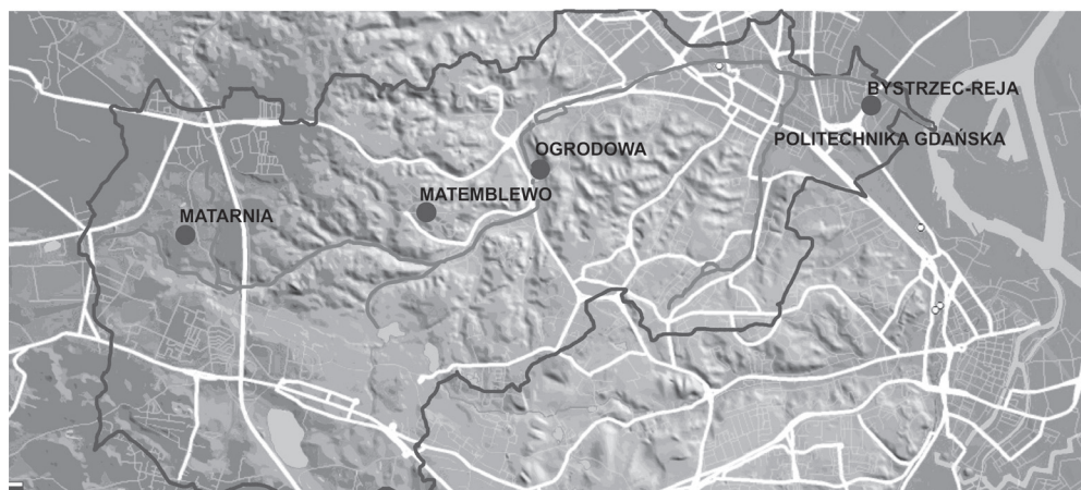
Fig. 2. Digital terrain model (DTM) of the Strzyża Stream catchment area with catchment boundary and precipitation gauges: Politechnika Gdańska - Gdańsk University of Technology - GUT (light point), Gdańskie Wody (circle) [12].
