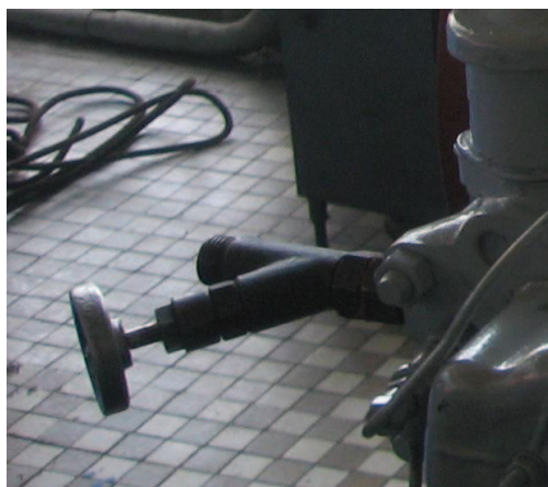
Fig. 2 Indicator valve installed in a place of holder of ignition paper (a) an electronic indicator PREMET C on a laboratory stand (b)
