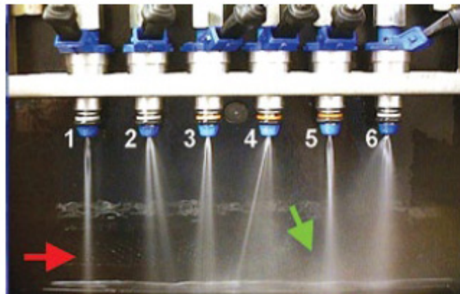
Fig. 7. Picture of the possible disturbances of the injectors' performance – a set of the same engine [www.intercars.com.pl]
