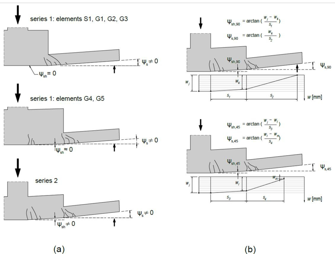
Fig. 14. Scheme of slab-column element deformation (a), Method for calculating the angle of rotation (b).
