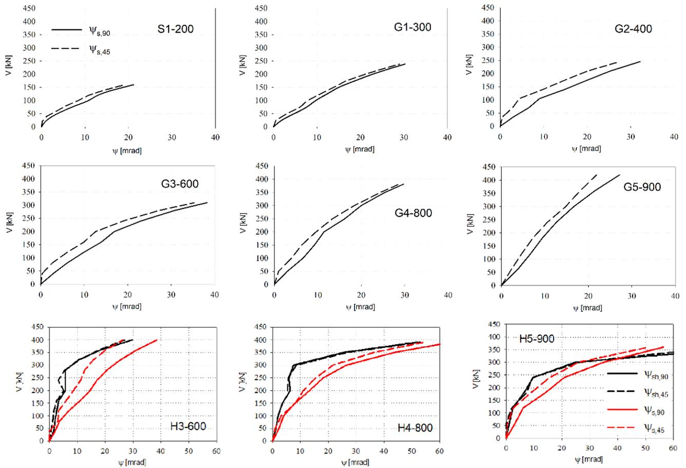
Fig. 15. Load-angle diagrams.
