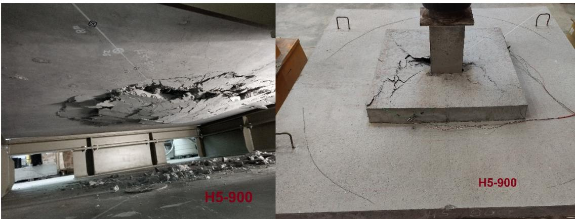
Fig. 11. Failure form of H5-900 element.
