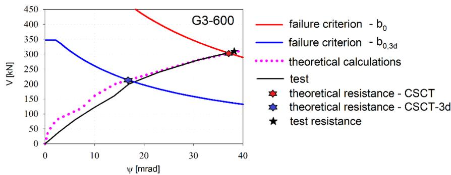
Fig. 16. Load capacity estimation using the CSCT method.
