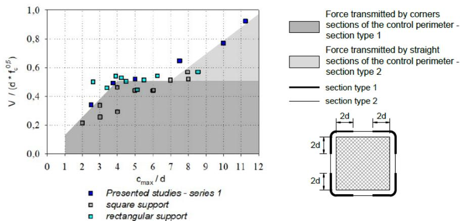
Fig. 21. Ultimate force depending on the parameter  $c_{max}/d$ . Interpretation of results.
