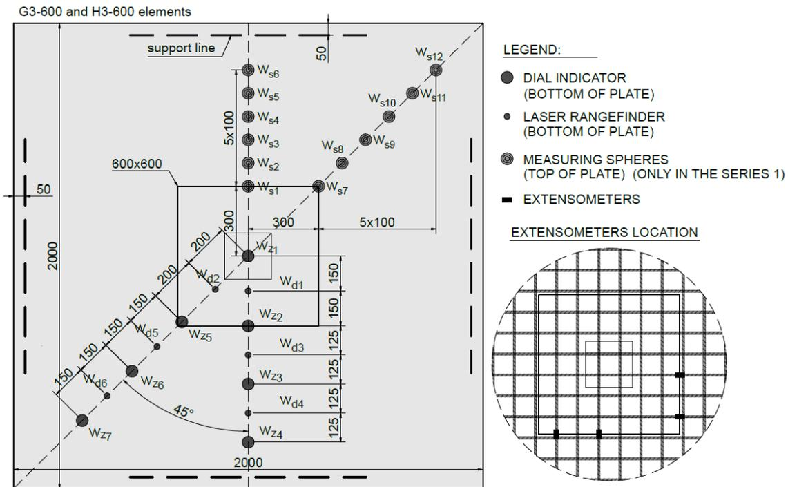
Fig. 6. Measuring points for G3-600 and H3-600 test elements.
