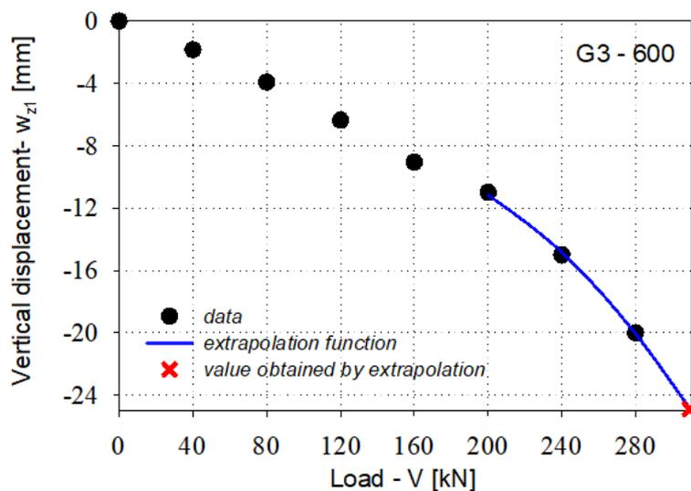
Fig. 7. Displacement extrapolation - element G3-600, measuring point  $w_{z1}$ .
