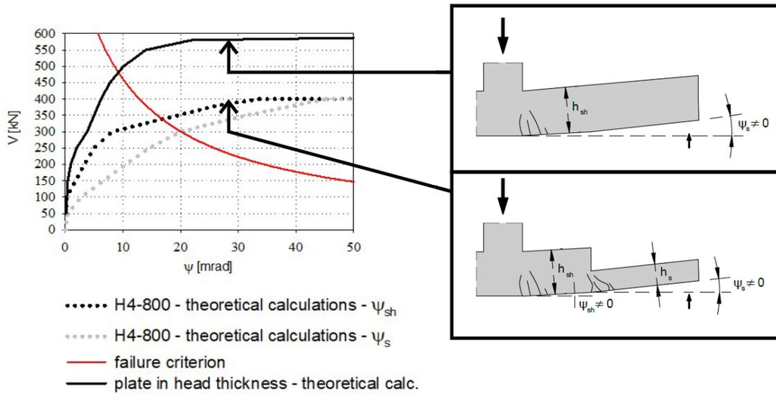
Fig. 18. Comparison of the behaviour of the element with and without drop panel according to CSCT calculations.
