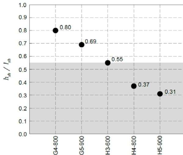
Fig. 19. Effect of head stiffness on failure mechanism.
