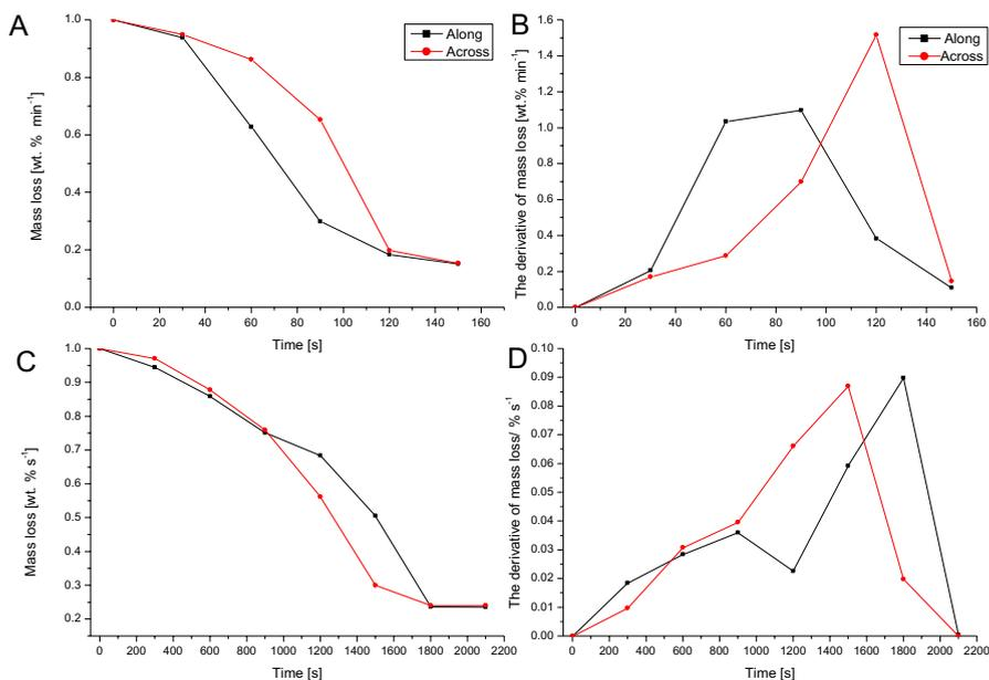
**Fig. 3** The pyrolysis process dynamic for particles with fibres oriented across and along the heat source: **A** and **B**. 20×20×5 mm samples (not insulated) and **C** and **D**. 32×30×30 mm samples (insulated on 5 walls)
