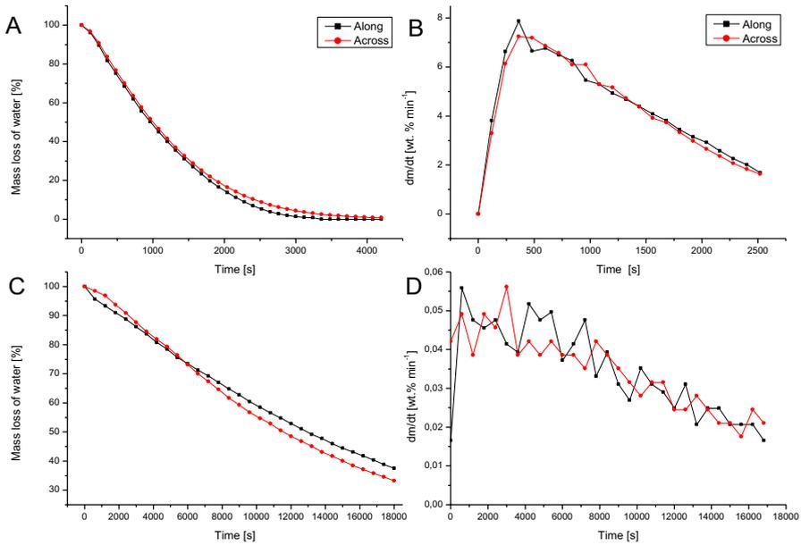
**Fig. 1** Experimental data of drying process dynamics for particles with fibres oriented across and along the heat source: **A** and **B** AC and AL samples with a size of  $20 \times 20 \times 5$  mm (not insulated) and **C** and **D** IAC and IAL samples with a size of  $32 \times 30 \times 30$  mm (insulated on 5 walls)
