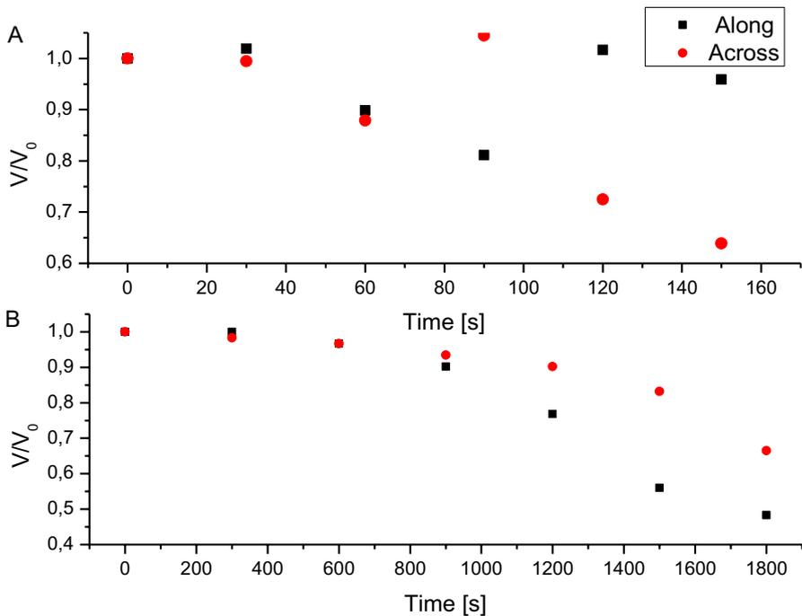
**Fig. 4** Change in volume of the samples during the pyrolysis process: **A.**  $20 \times 20 \times 5$  mm samples (not insulated) (AC and AL) and **B.**  $32 \times 30 \times 30$  mm samples (insulated on 5 walls) (IAC and IAL)
