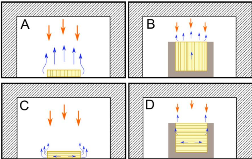
**Fig. 2** Heat and flow distributions during the drying process for samples with fibres oriented across the heat source: **A**. AC and **B**. IAC. Heat and flow distributions for samples oriented along the heat source: **C**. AL and **D**. IAL (arrows pointing from top to bottom- heat distribution; arrows pointing from bottom to top- steam)
