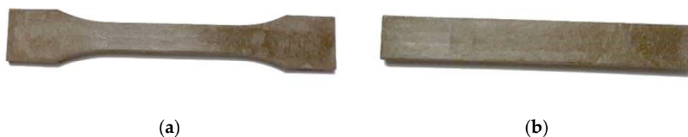
Figure 1. Specimens for: (a) tensile test; (b) bending test.
