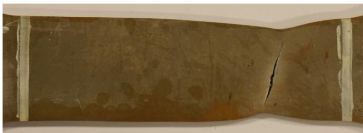
6.5 specimen – FE (top) and experimental (bottom) failure mode
