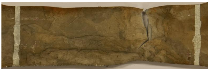
8.1 specimen – FE (top) and experimental (bottom) failure mode
