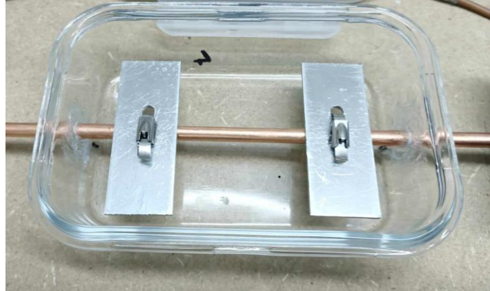
Fig. 2. Aluminum fins added inside PCM container.
