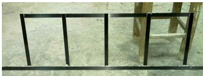
Fig. 3. Reinforcing cage before covering with sand
