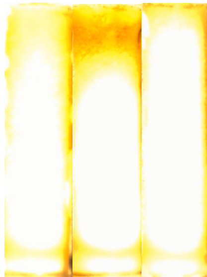
Figure 13. Solidification front images for different geometry of storage units but for the same process time equal to 35 min and the same constant wall temperature condition ( T_s = 17\text{ }^\circ\text{C} ): at left for annular TES, at the middle for shell-and-coil TES with coil position at the bottom of the tank, at the right for shell-and-coil TES with coil position at upper of the tank.
