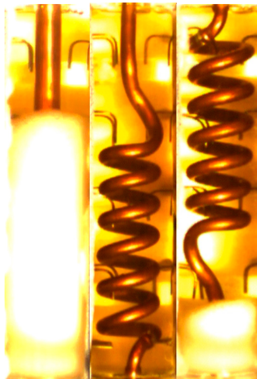
Figure 19. Melting front images for different geometry of storage units but for the same process time equal to 90 min and the same constant wall temperature condition ( T_s = 34\text{ }^\circ\text{C} ): at left for annular TES, at the middle for shell-and-coil TES with coil position at the bottom of the tank, at the right for shell-and-coil TES with coil position at upper of the tank.
