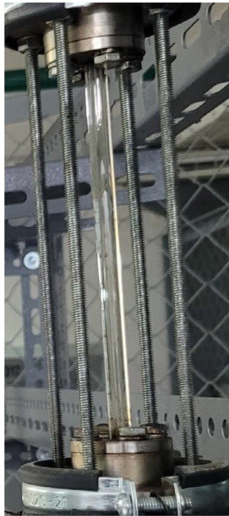
Fig. 5. Visualization test section – borosilicate glass tube, d_{in} = 3 \text{ mm} , l = 100 \text{ mm} .
