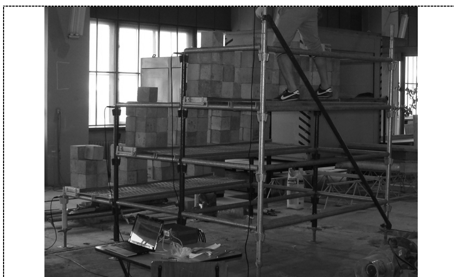
Figure 1. Steel temporary grandstand with typical diagonal stiffener.
