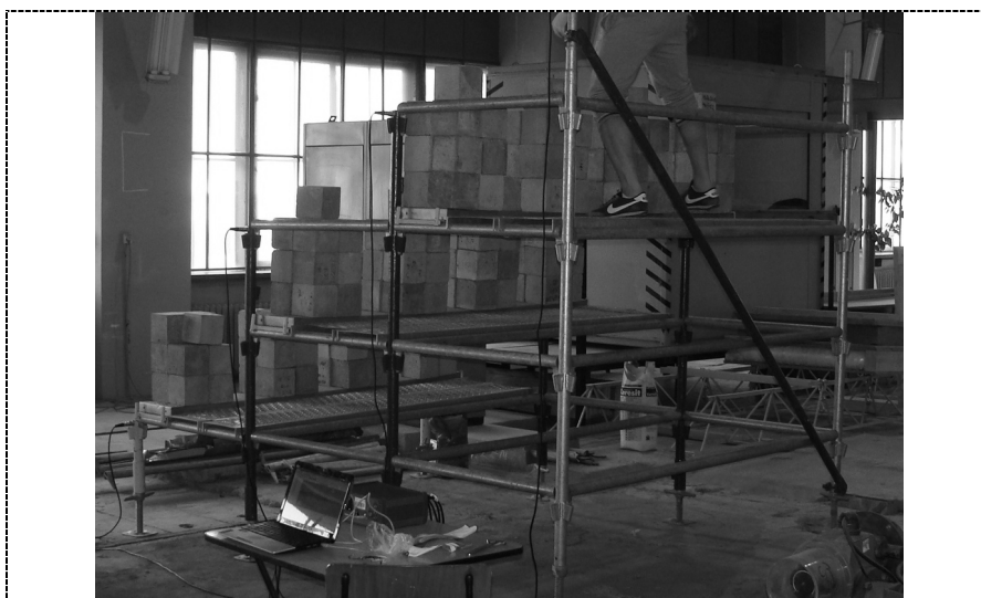
Figure 1. Steel temporary grandstand with typical diagonal stiffener.
