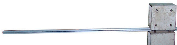
Figure 9. Aluminium cantilevered composite beam.
