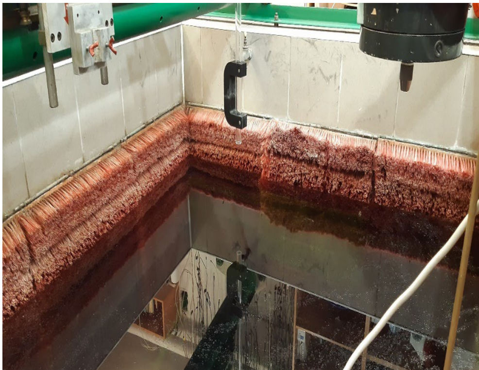
Figure 1. Damping curtains with plastic brushes in the tank of the Department of Sonar Systems GUT.
