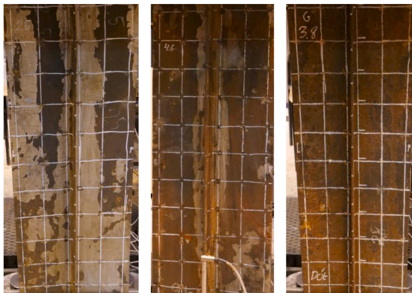
Fig. 3. Corroded stiffened plates: 2.5 mm (left); 4.6 mm (mid); 3.8 mm (right) (Woloszyk et al., 2021b).
