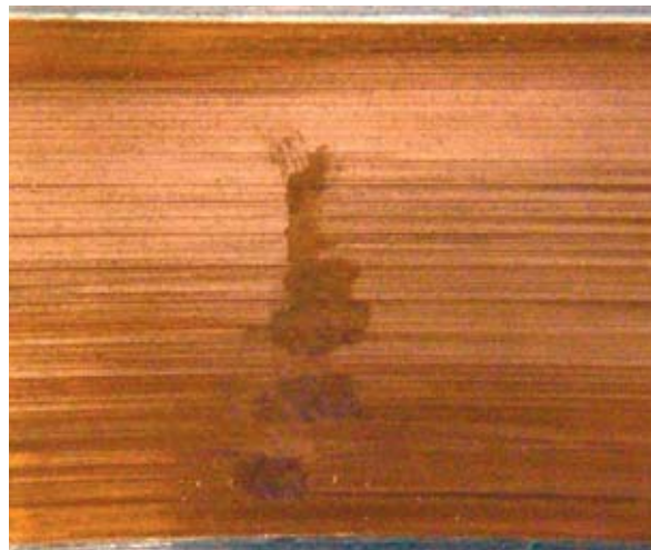
Fig.3. Fatigue cracks on the slide bearing surface for the alloy MB11, obtained after the test on SMOK stand
