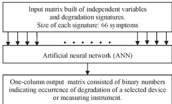
**Fig. 3.** Inputs and outputs of one ANN (out of 37 dedicated ANNs) dedicated to fulfil role of a diagnostic relation which identifies degradation of one, out of 22 (see Tab.1), geometrical dimension of component devices of steam power unit or one, out of 15, (see Tab. 1, items No. 23 through 37), measuring instrument located at the cycle's extractions.
