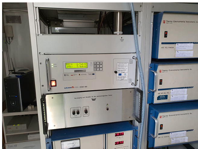
Fig. 7. Equipment for reference PM measurement (Gimm 180 analyser) installed in the reference Station 3 of ARMAG foundation.
