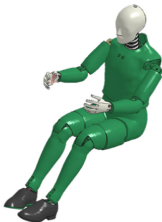
Figure 3. FE model of a 50 th percentile Hybrid III male dummy.
