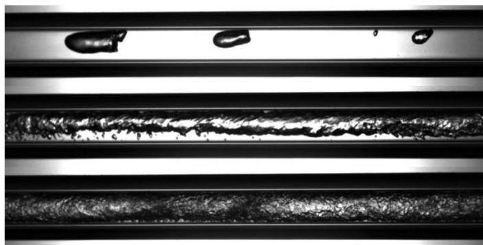
Figure 7.1 Flow structures of R1233zd(E) in 3mm horizontal pipe under saturation temperature 83°C, saturation pressure 0.71 MPa, reduced pressure p_r=0.2 , and mass velocity 1000 kg/(m 2 s)
