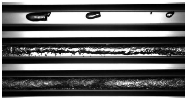
Figure 4.18 Flow patterns of R1233zd(E) in 3mm horizontal pipe under saturation temperature 83°C, saturation pressure 0.71 MPa, reduced pressure p_r=0.2 , and mass velocity G=1000 \text{ kg/(m}^2\text{s)} . Quality respectively: 0.67% 5.9% 24.3%
