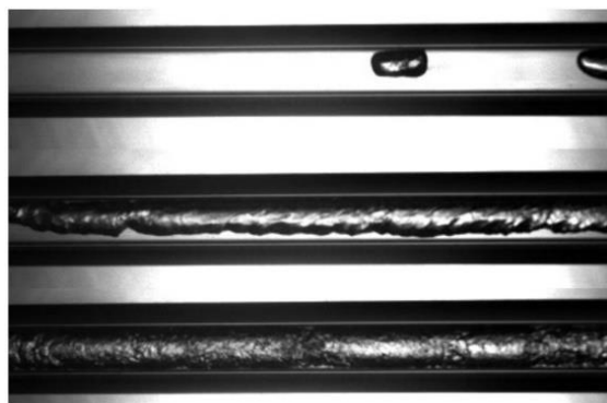
Figure 4.19 Flow patterns p_r=0.2 G=600 \text{ kg/(m}^2\text{s)} Quality respectively: 1.13% 10.47% 30.02%
