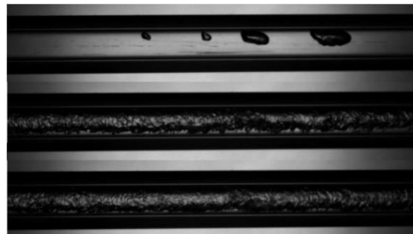
Figure 4.20 Flow patterns p_r=0.4 G=600 \text{ kg/(m}^2\text{s)} Quality respectively: 2.54% 31.11% 38.15%
