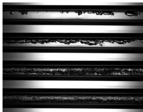
Figure 4.21 Flow patterns p_r=0.6 G=600 \text{ kg/(m}^2\text{s)} Quality respectively: 3.17% 8.91% 30.23% 49.73%
