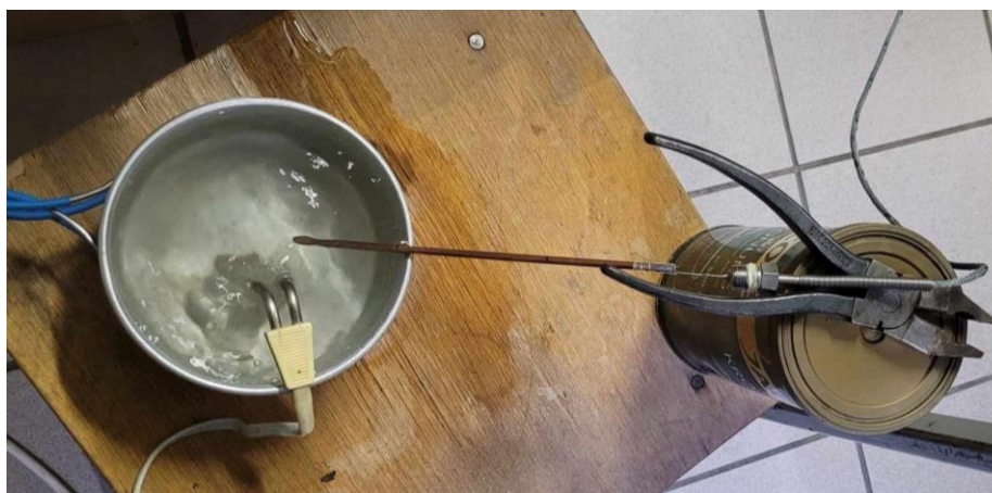
Figure A4.1 Experimental setup – boiling water, examined 200 mm long copper tube with thermocouple K attached 10 mm before the end of the tube.
