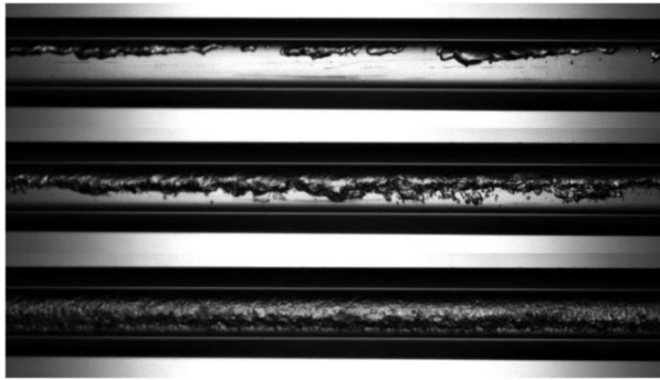
Figure 4.22 Flow patterns p_r=0.7 G=600 \text{kg}/(\text{m}^2\cdot\text{s}) Quality respectively: 2.45% 15.86% 45.10%.
