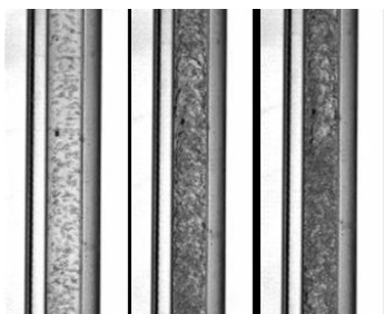
Figure A6.5 Flow patterns p_r=0,8 G=355 \text{kg}/(\text{m}^2\cdot\text{s}) , quality respectively: 8,2%, 19%, 33,7%.
