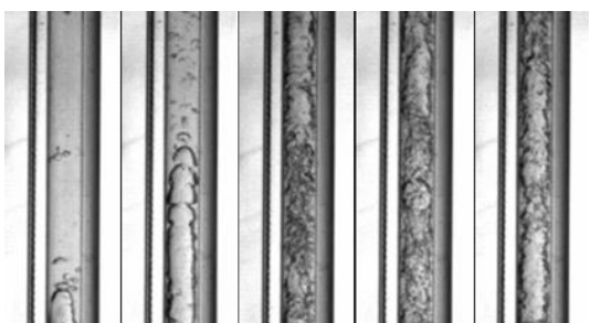
Figure A6.6 Flow patterns p_r=0,6 G=180 \text{kg}/(\text{m}^2\cdot\text{s}) , quality respectively: 37,2%, 48,6%, 64,6%, 72,8%, 93%
