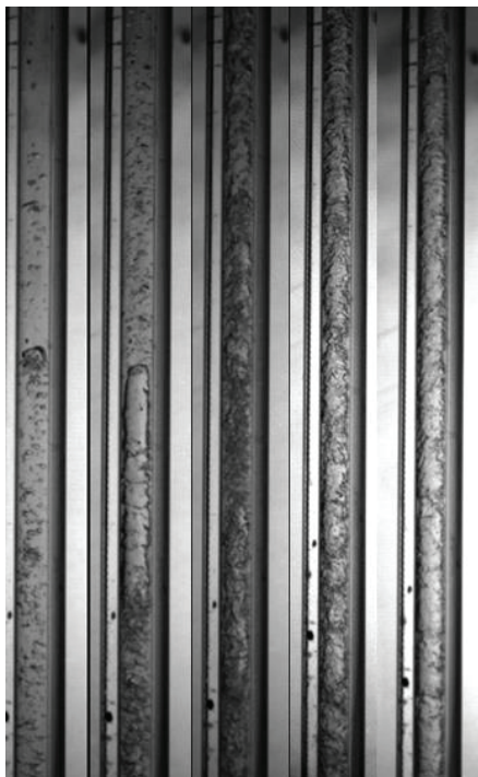
Figure 5. Flow Patterns Pr=0,6 G=355 \text{kg}/(\text{m}^2\cdot\text{s}) Quality respectively: 12%, 15,6%, 19,6%, 23,9%, 36,2%, 60,7%
