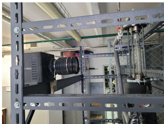
Figure 2. The visualization section with the Photron Fastcam Mini UX100 high-speed camera. Behind the visualization section is an led light source.
