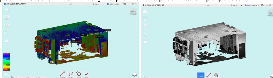
Figure 3: Performing the tasks phase 1 - clearing, measuring elements of cloud, ReCap
