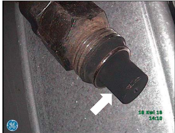
h) Fuel injector removed from the cylinder head – thick layer of soot on the spray tip
