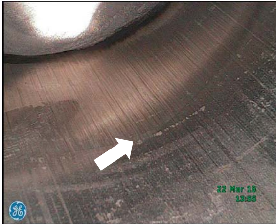
a) Cylinder surface in the lower part of the liner – traces of abrasive and erosive wear, no visible traces of honing of the liner
