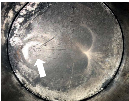
Cylinder liner closed by the piston head – clean surface, identification numbers visible
