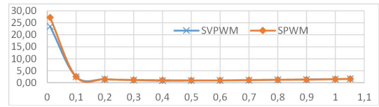
Fig.23. The comparison of a phase voltage THDs of proposed SVPWM and SPWM with common-mode voltage injection when generating only the first output voltage harmonic (50Hz). The modulation indexes vary from 0.01 to 1.0515. Results of experimental tests.
