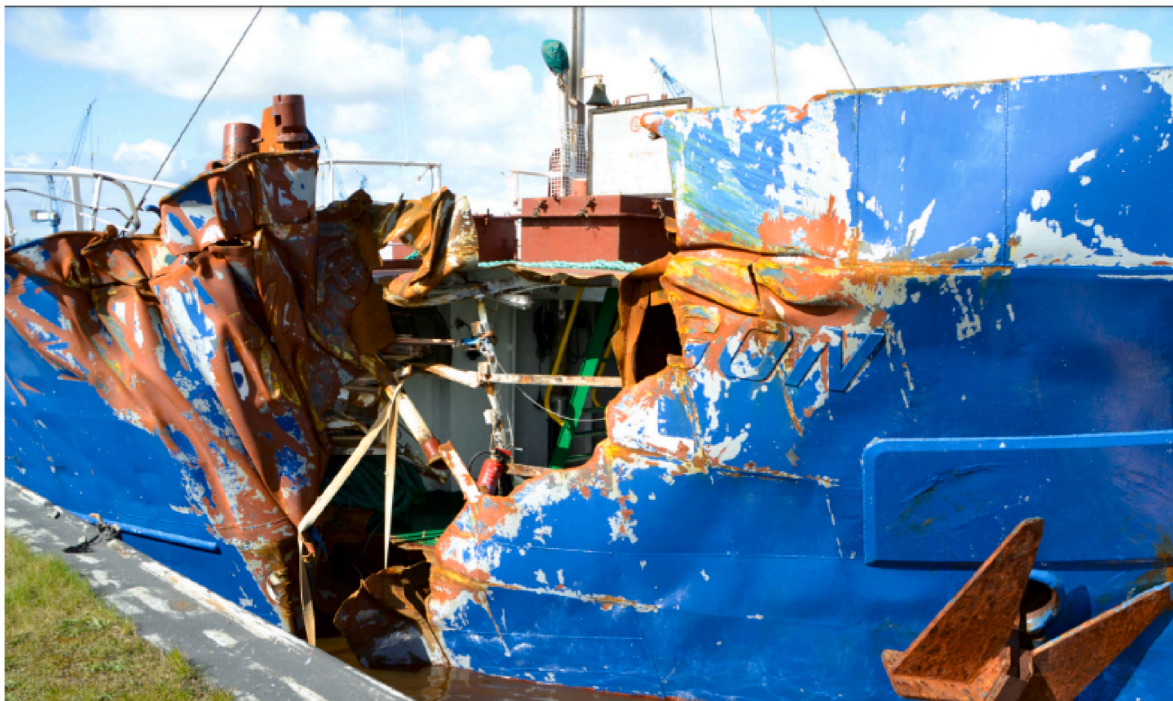
Fig. 2. Collision damage of the ship Petra L. (LOA = 74m) on the Gode Wind 1 offshore wind farm (monopiles D = 6m, 6 MW) (Mandra, 2023).
