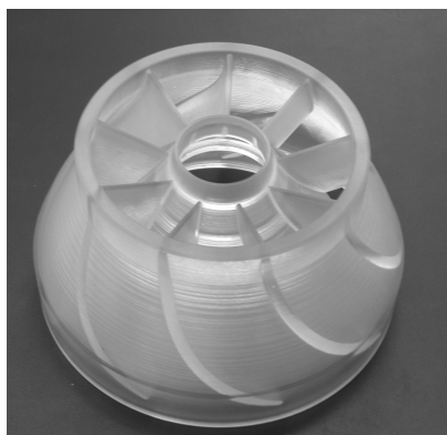
Fig. 2. Exemplary product (pump diffuser) developed with the use of Rapid Prototyping Technology
