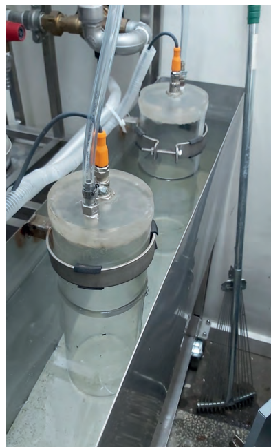
Fig. 3. Biogas collecting vessels with gas throughput sensors
