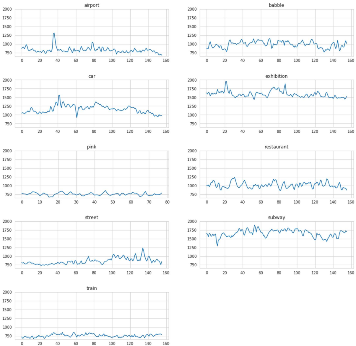
Figure 4.36 Spectral centroid of noise recordings
