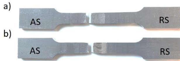
Fig. 12 Fracture locations of the welds produced with the tapered cylindrical pin (a) and the hexagonal pin with grooves (b)
